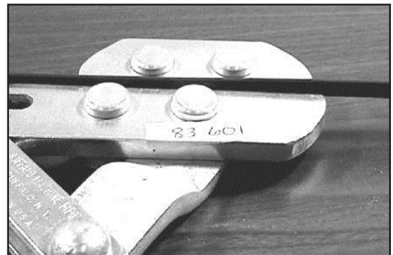
Buffalo Grip for tensioning cable. Note Grip jaws are only on the steel support strand.
