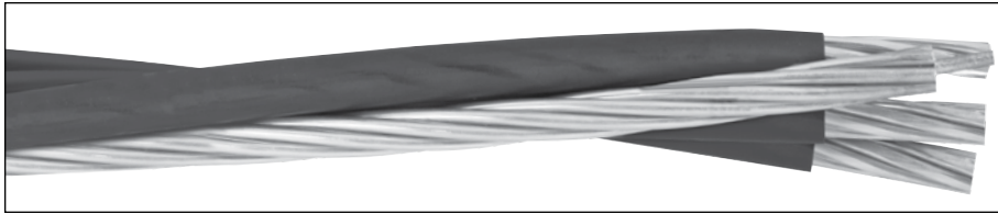
QUADRUPLEX TYPE NS75/NS90 – XLPE – ACSR FULL SIZE NEUTRAL – 600 VOLTS
